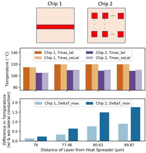
**Figure 6: Top view of the upper tier with 10% hot spot area. Chip 1 contains lumped hot spots, while chip 2 contains scattered hot spots. The graphs show maximum on-chip temperatures and significance of lateral heat flow modeling in chips 1 and 2.**
